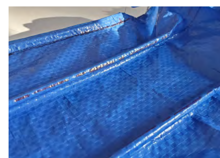
EMBEDDED STICK MOD: Adding stiffness to the polypropylene surface
