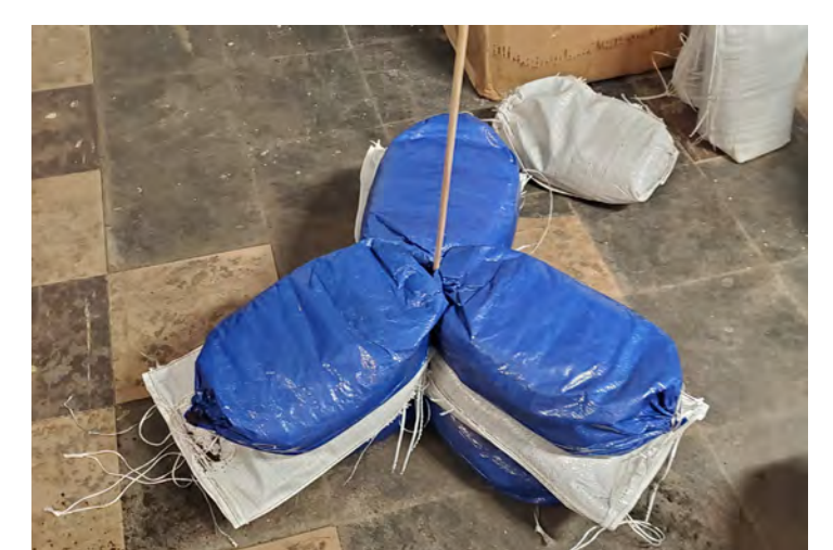
CORNER-STITCH TRI STACK: 3 courses vertically joined with a center dowel
