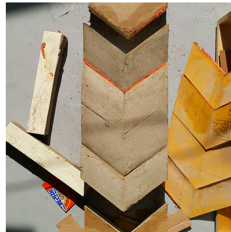
FIGURE 3: UNCASTING THE CONCRETE PANEL. PHOTO: M. SHAFFER
