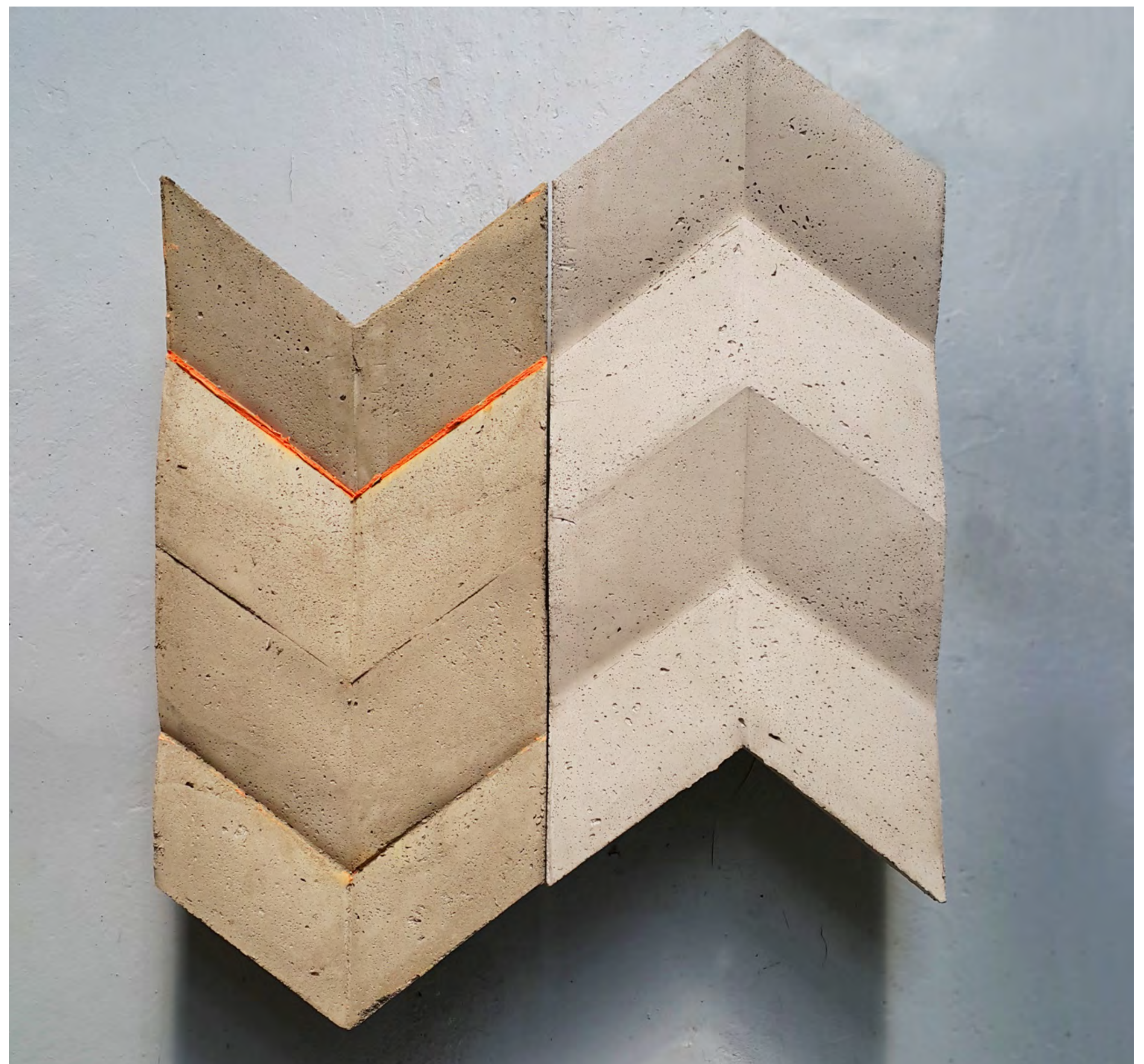
FIGURE 4: FINISHED PANELS AFTER UNCASTING. PHOTO: M. SHAFFER
