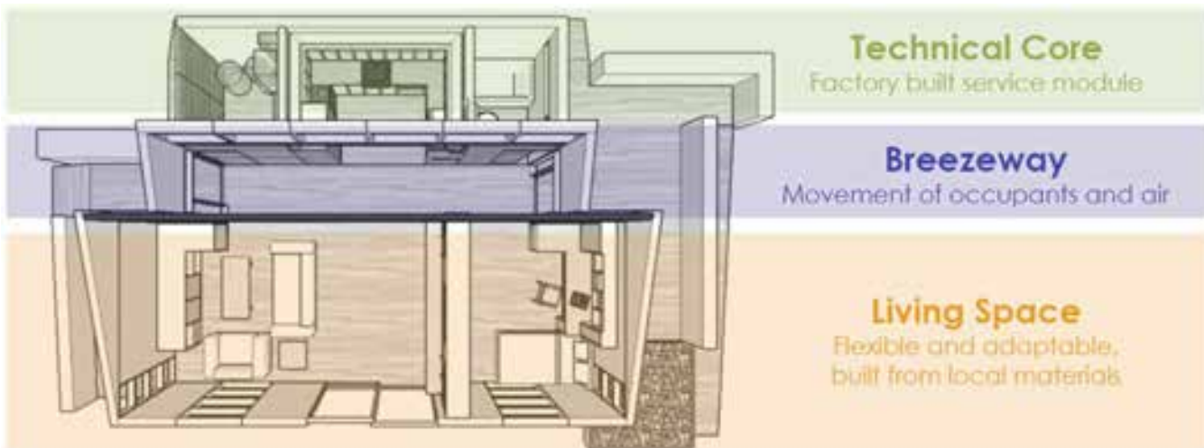
Fig. 1: Diagram of three basic components of the MorningStar home
