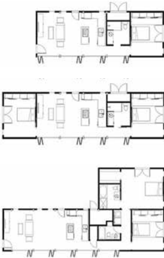
Fig. 5: Plans of Natural Fusion "Get Ready to Own (gr2o)". Prospective owners could purchase a home using an interactive website choosing from three configurations; base module (top left), two-bedroom versions (middle and bottom plan). (Courtesy of the 2009 Penn State Solar Decathlon Team)
