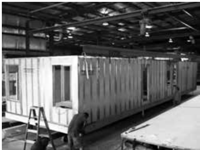
Fig. 8: EEHP modules on the assembly line in the modular home manufacturing plant. (Photograph by author)
