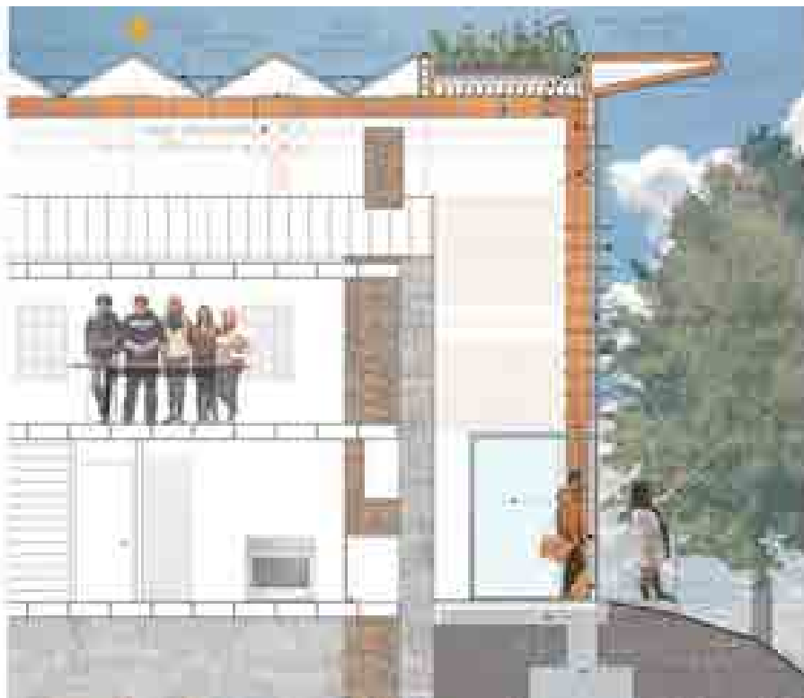
New Wall Section This section shows the meeting of various reclaimed and high efficiency materials.
