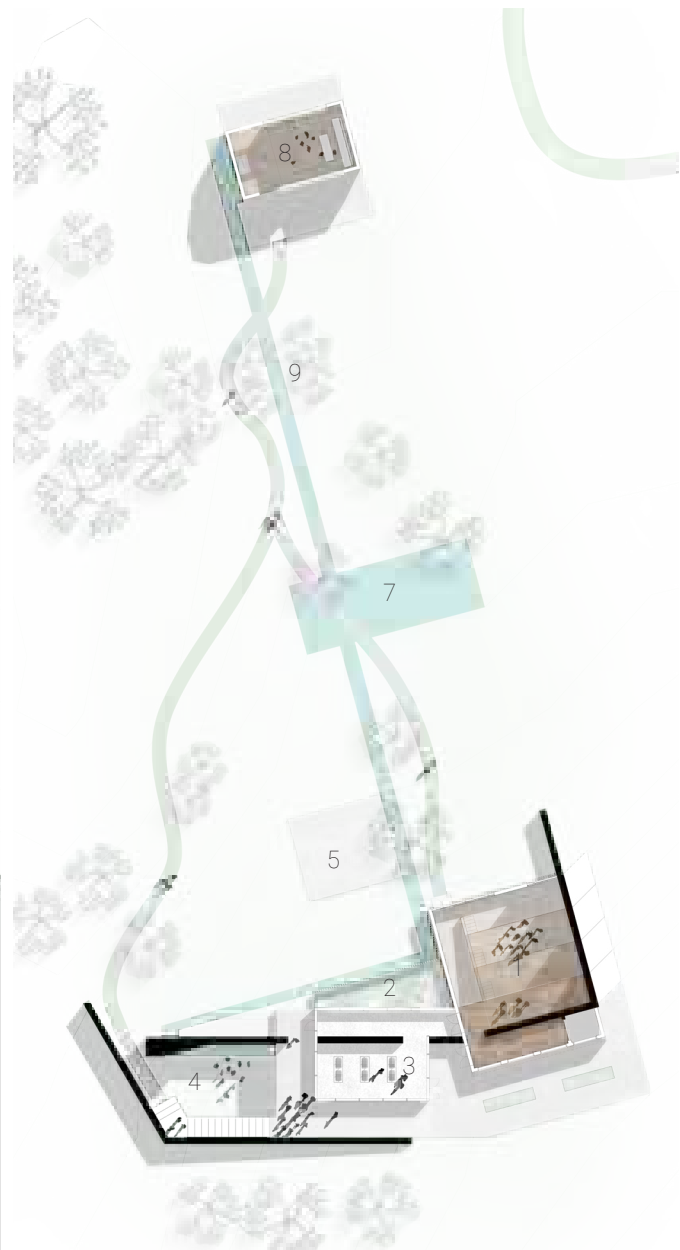
Upper plan of new building and farmhouse showing the kitchen, classrooms and greenhouse and the relationship between the two structures.
