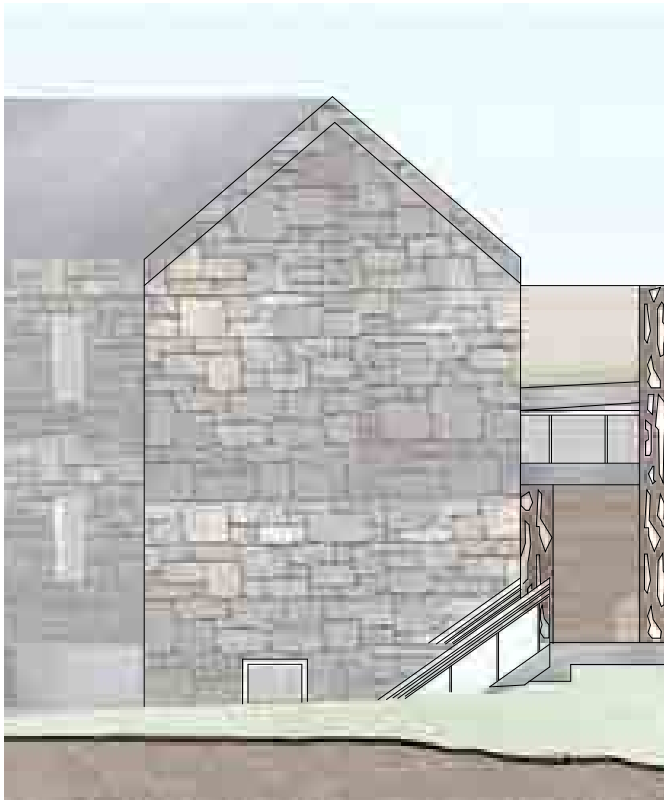
Side Elevation This elevation emphasizes the meeting point of the existing stone walls of the farmhouse and the new materials of the addition. These materials include wood clad walls, metal screens and a green roof.
