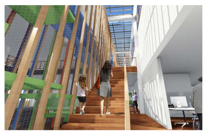
**Rendering of Spine During Day** The glass core creates a bright, playful circulation space. The addition of the wooden slats prevents too much direct light from entering the space and overwhelming occupants with harsh lighting.
