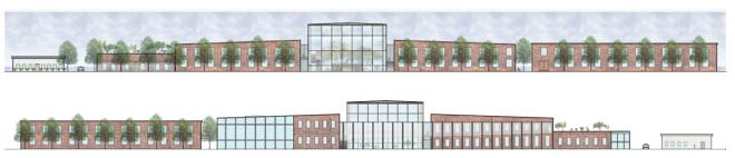
Above are two elevations displaying the north and south facades. The north facade depicts the view from High Street, as well as the brick veneer and glass materials used. Trees form a wall for natural air cooling on the northern facade. The glass-covered trail, which provides a buffer zone between the interior of the facility and exterior, is seen on the south facade.
