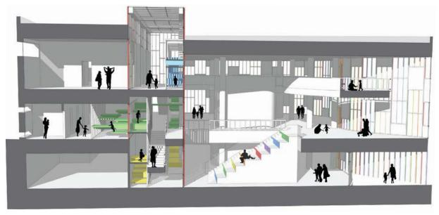
**Transverse Section** This section show off the duality of the building, bisected by the circulation spine. Also visible are the climbing platforms, which are color-coded by floor.
