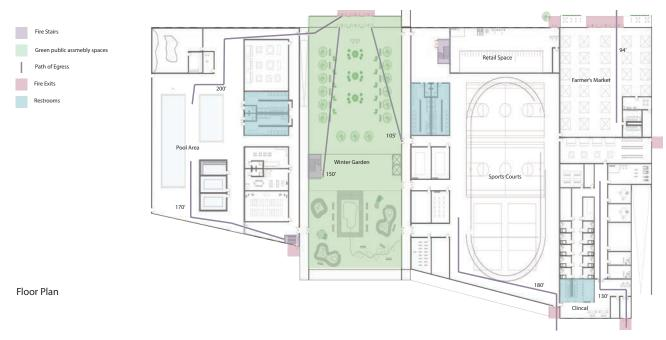
The presence of a central, continuously accessible greenspace encourages community cohesion through engagement with adjoining fitness spaces. These spaces are made accessible by fire exits, stairwells, and elevators.
