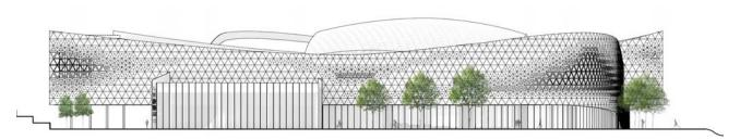
**South Elevation** This view faces King St, one of the main roads into Pottstown. The facade is formed from triangulated metal paneling that wraps around the building, peeling up to expose the entrances.
